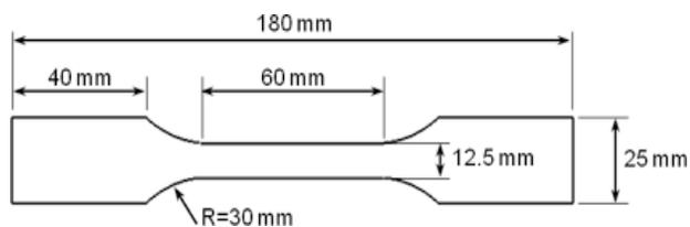
Figure 1: Tensile test specimens
