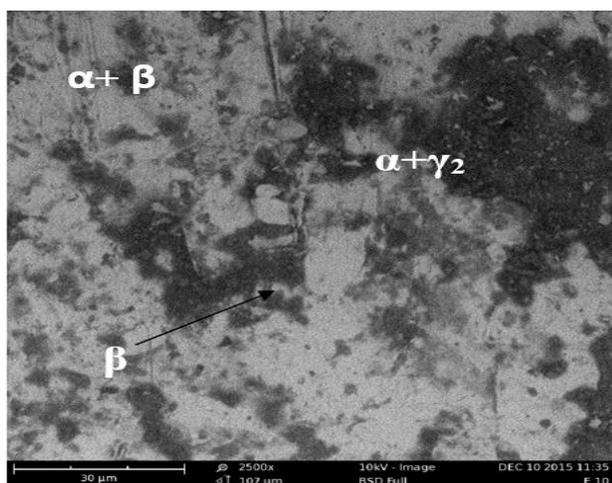
Figure 6: Plate 24: SEM micrograph of Cu-10%Al + 10%Mn
