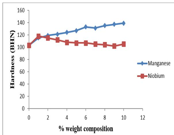
Figure 9: Effect of alloy compositions on the hardness of aluminium bronze (Cu-10%Al)
