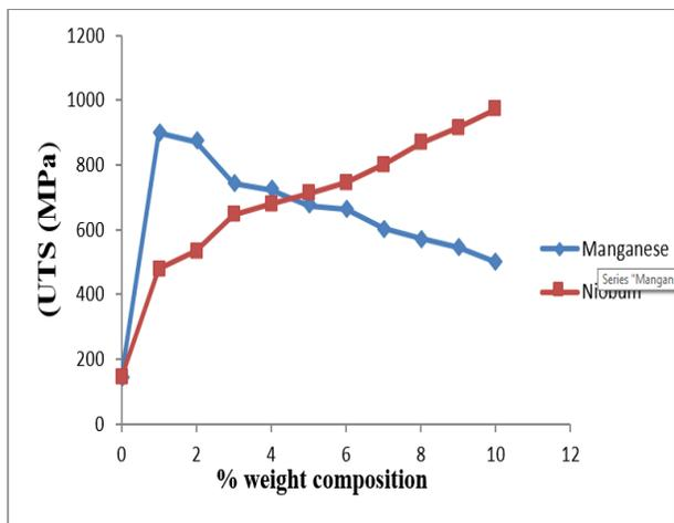
Figure 7: Effect of alloy compositions on the UTS of aluminium bronze (Cu-10%Al)
