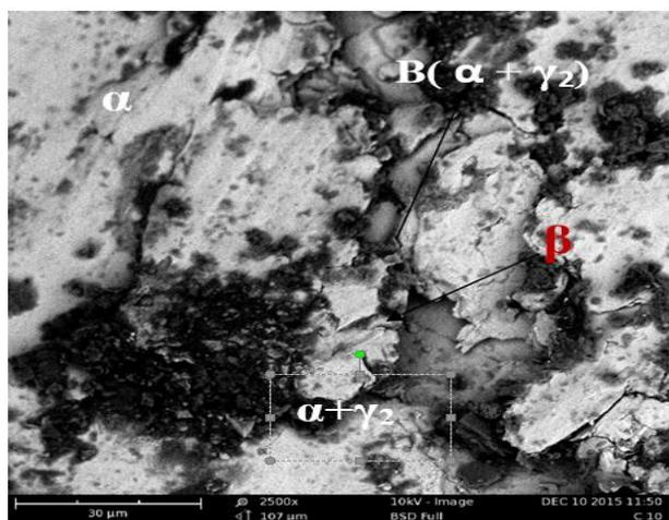
Figure 4: Plate 22: SEM micrograph of Cu-10%Al
