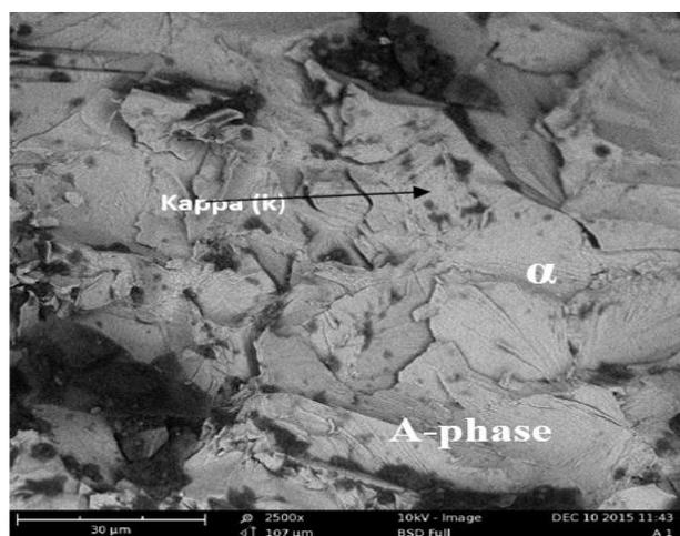
Figure 5: Plate 23: SEM micrograph of Cu-10%Al + 10%Nb (X2500)
