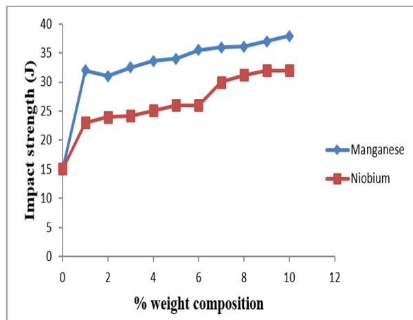
Figure 10: Effect of alloy compositions on the impact strength of aluminium bronze (Cu-10%Al)
