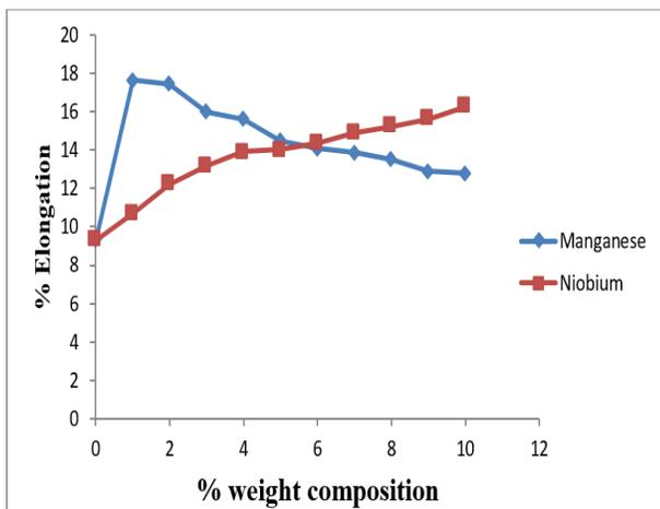
Figure 8: Effect of alloy compositions on the % elongation of aluminium bronze (Cu-10%Al)
